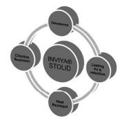
INVIYA STOLID is variant of INVIYA's I-400 and this proprietary polymer has high power, which leads to lasting fit & shape retention, it is resistant to heat & dyes with Polyester at 130 degrees. Apart from this, this is chlorine resistant making it suitable for swim wear/beach wear.
